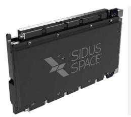
FeatherEdge<sup>™</sup> Gen. 3 is a 3U VPX Single Board Computer aligned to the Sensor Open Systems Architecture (SOSA) standard which ensures seamless integration with SOSA-aligned systems.
