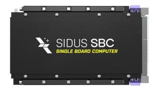
The Sidus Single Board Computer (SSBC) is a rugged, modular 3U VPX solution designed for size-constrained and mission-critical applications and engineered for high-performance computing in extreme environments.
